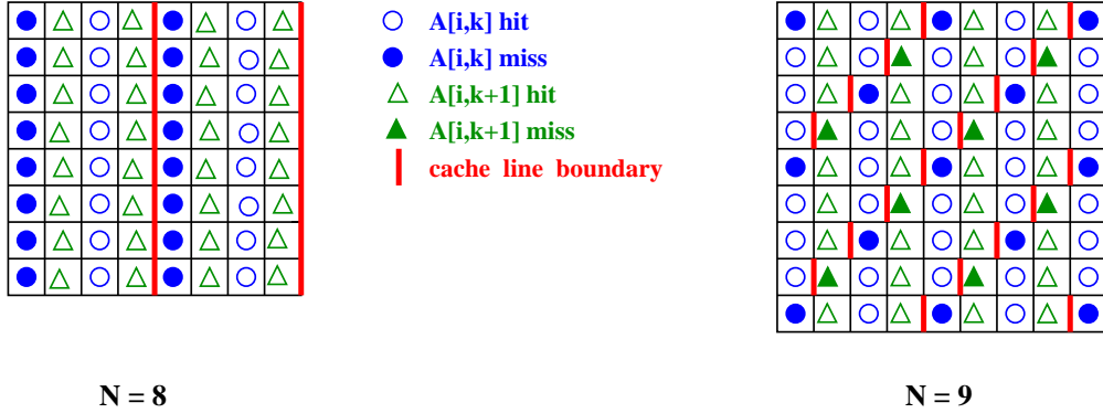
Figure 2: The distribution of cache misses for the two references to matrix A from the matrix multiply code presented in Figure 1, for an even problem size ( N=8 ) and an odd problem size ( N=9 ), assuming an architecture with a cache line that holds four double elements.
